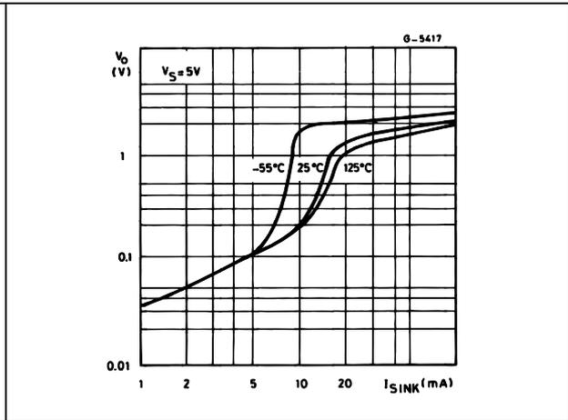
Figure 7. Low output voltage versus output sink current
