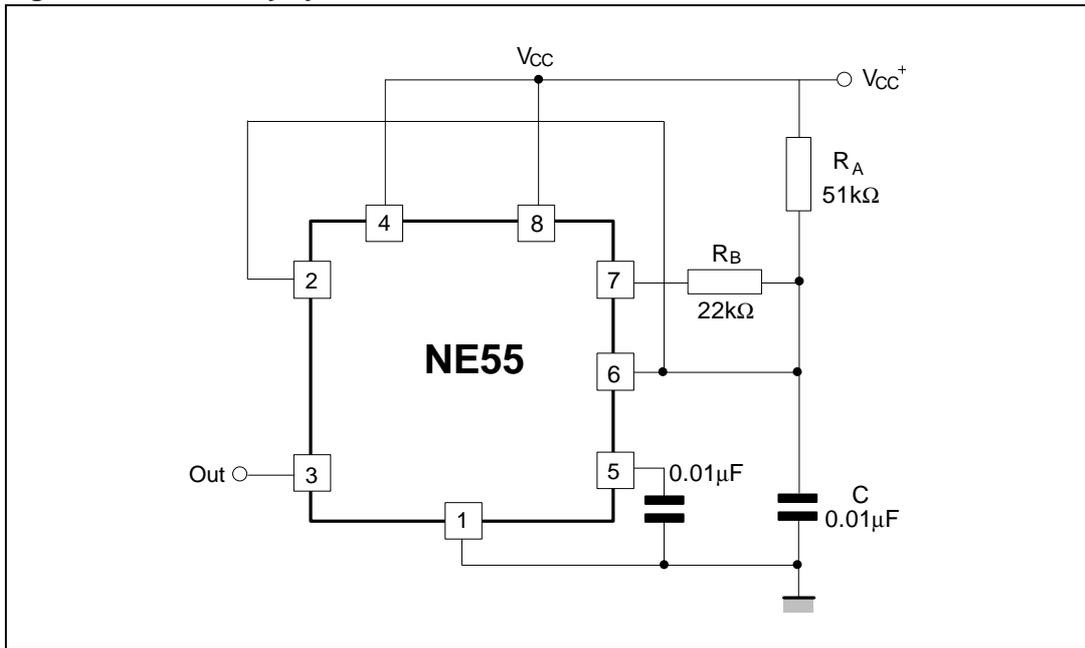
Note that this circuit will not oscillate if  $R_B$  is greater than  $1/2 R_A$  because the junction of  $R_A$  and  $R_B$  cannot bring pin 2 down to  $1/3 V_{CC}$  and trigger the lower comparator.
