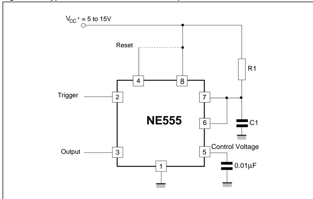
The circuit triggers on a negative-going input signal when the level reaches  $1/3 V_{CC}$ . Once triggered, the circuit remains in this state until the set time has elapsed, even if it is triggered again during this interval. The duration of the output HIGH state is given by  $t = 1.1 R_1 C_1$  and is easily determined by [Figure 14](#).
