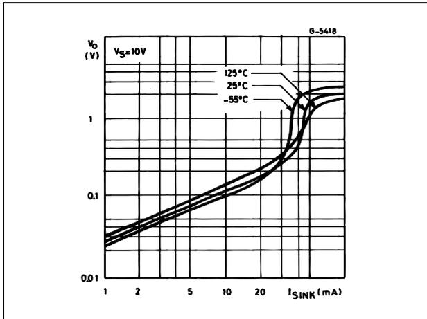
Figure 8. Low output voltage versus output sink current
