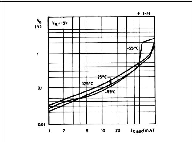
Figure 9. High output voltage drop versus output
