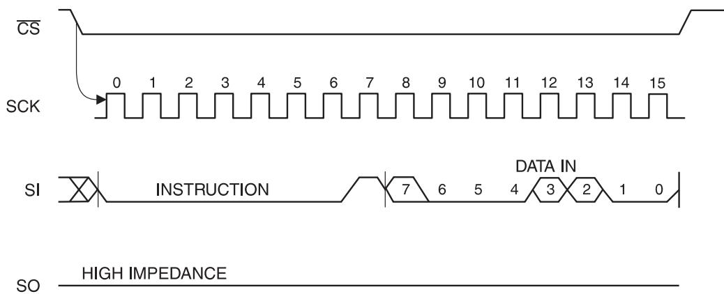
**Figure 8.** READ Timing
