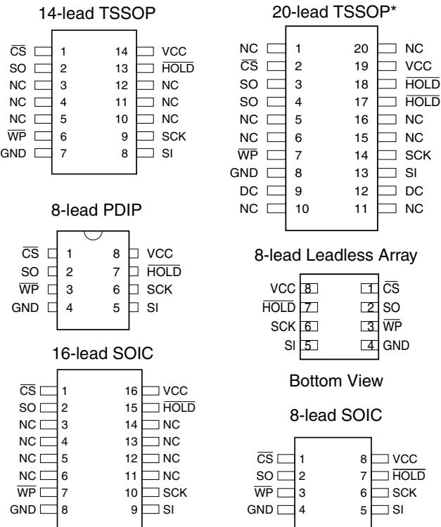
\*Note: Pins 3, 4 and 17, 18 are internally connected for 14-lead TSSOP socket compatibility.
